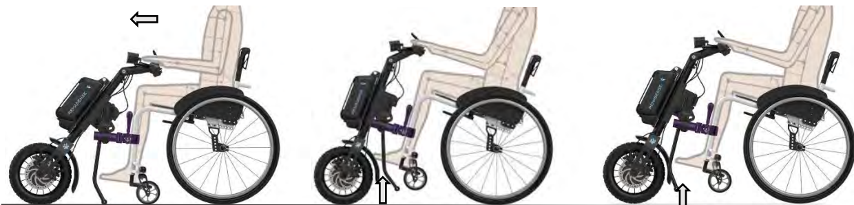
Figure 36. Parking (1), City (3) and Touring (2) positions for Manual Clamp/Lift Devices
