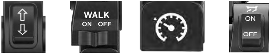
Figure 39. Switches and Indicators (L to R) Direction; Walk; Cruise; Traction
