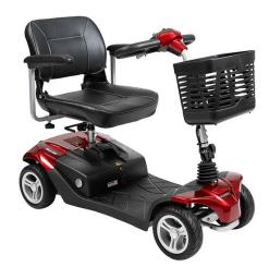
**Pull-Apart Aluminium Frame Designed to Maximise Mobility.** This lightweight medium sized scooter is designed for ease of transport in a car. Packed with category leading features, it is highly capable outdoors offering a 39 km range.
