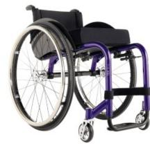
Using special techniques such as welding, the Küschall-Team have made the sleek and dynamic design of The KSL priority, not only keeping unseemly parts to a minimal but reducing the weight of the chair to in its standard configuration to less than 7kg.
