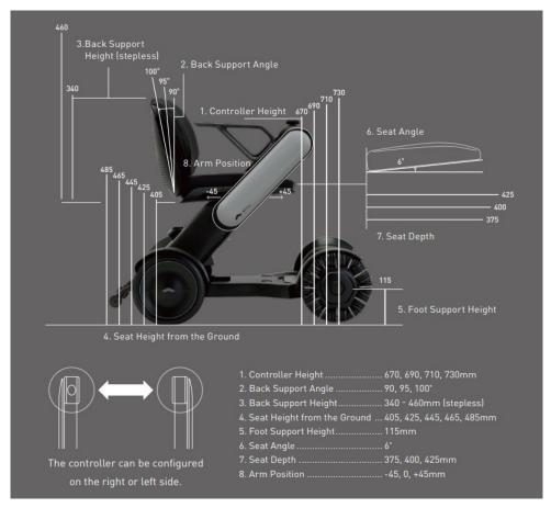
Model Ci can be easily adjusted from seat height and back support angle to controller position (right or left drive) to create a comfortable driving experience.
