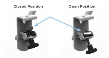
2. With both hand wheels now unscrewed, lift the rail into position. It is important that the rails are fitted to a specific position on the bed, which is indicated by the bolt on top of the bed frame. Position the rail over the bolt and tighten the hand wheel to the closed position.
