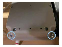
2. Use your flat object to unlock the control box case as shown.
