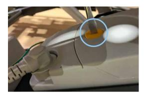
3. Locate the correct port for the battery backup and remove the rubber plug.
