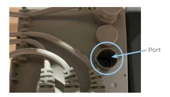
4. Plug the battery backup into the port and replace the cover.
