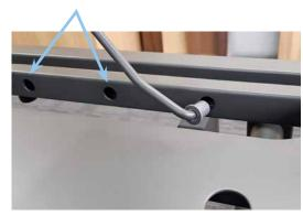
To extend the mattress retainer hold vertically and insert ends into 1 of the 3 receiving keyhole mounts which are 100mm spaced at the foot end of the mattress platform to match the desired bed extension (nil, 100mm, 200mm). Lower the retainer to the mattress platform. It will now be locked in place at the mount keyholes.
