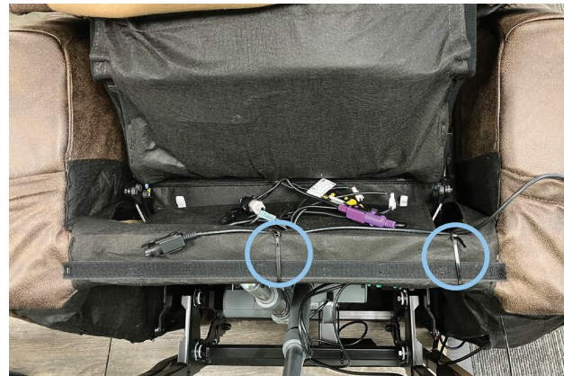
4.4.6 Attach the extension cable to the base frame using cable ties as shown
