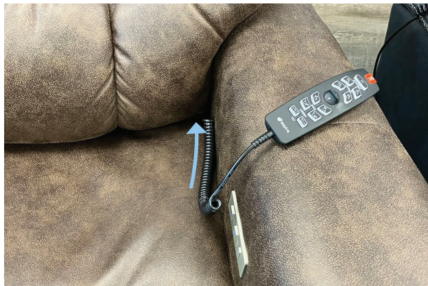
4.4.7 Feed the handset cable through the back of the left hand side armrest towards the back of the frame
