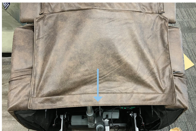
4.4.9 Cover the back of the frame with the frame covering / curtain
