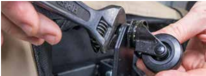
4.3.2 Attach castor stem through plate, lock in place with retaining nut
