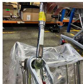
3. Use a torque wrench to tighten the pintle bolt to 25-28Nm
