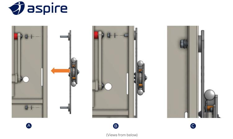
4. A B Insert rail into bed mounting holes. Ensure that the bed spacers are present and in position as shown
