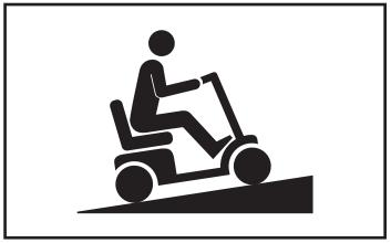
Figure 4. Increased Stability Driving Position
