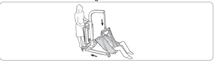
When lifting to the floor, the wheels of the lift should not be locked. When the patient touches the floor, the lift should be pulled backwards to give space for the head. **Tip:** If lifting is to a thinner gym mat, the lift can be pushed in under this mat, so that the mat acts as a soft protection between the lift and the patient. If the sling is to be removed, see "Removing the Sling when the Patient is Lying in Bed", page 11.
