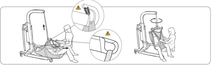
Smooth out the leg supports under the patient's legs. First connect the upper strap loops to the sling bar, then the leg support loops. See page 6-7 for instructions on how to attach the sling loops to different sling bars. Keep the leg supports away from the groin to prevent discomfort to the patient. This is facilitated if the patient bends the legs.
