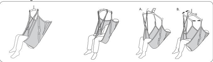
Soft Original HighBack Sling in **twopoint suspension** provides for a slightly reclined sitting posture with excellent head support and approx. 90 degrees angle in the hip joint.
