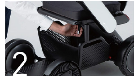
Raise the lever under the seat.
